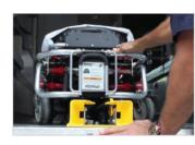
SAE J3027 compliant when combined with the Stat Trac® Cot Fastening System
