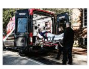
5-position drop frame provides better leverage for lifting and loading and reduces the cot length by 15 inches for movement in confined spaces
