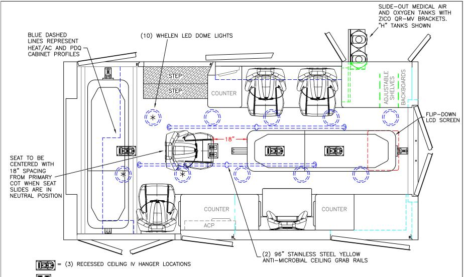
\* = (2) RADIO ANTENNA BASES LOCATED OUTBOARD OF DOME LIGHTS WITH COAX SERVICE LOOP (1) AM/FM RADIO ANTENNA FOR PATIENT COMPARTMENT RADIO
