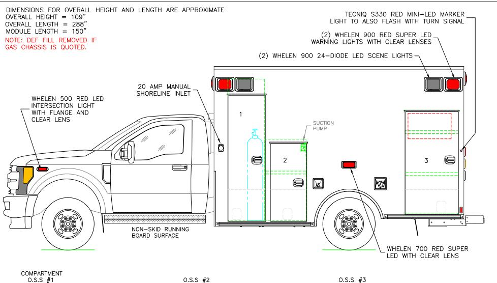
CLEÄR OPENING: 74.50h x 18.50w INSIDE DIM'S.: 84.75h x 22.00w x 18.50d OXYGEN STORAGE COMPARTMENT O.S.S #2
