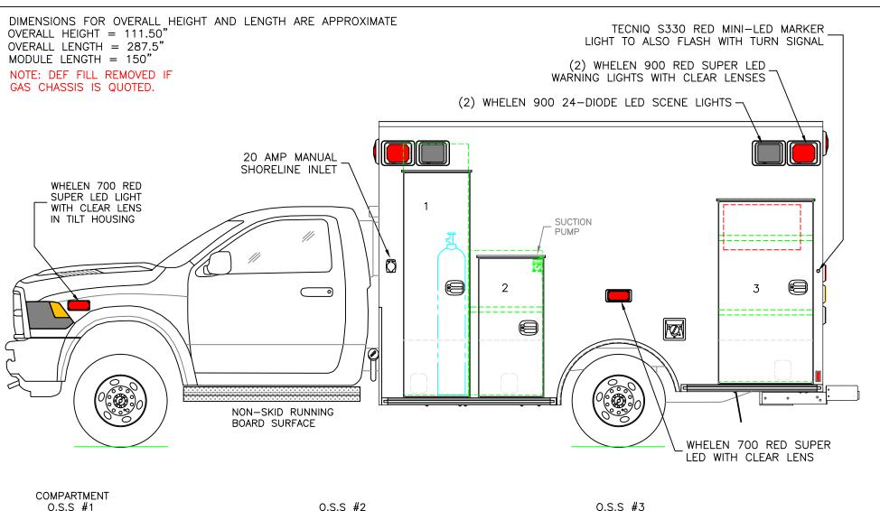
CLEÄR OPENING: 74.50h x 18.50w INSIDE DIM'S.: 84.75h x 22.00w x 18.50d OXYGEN STORAGE COMPARTMENT D.S.S #2
